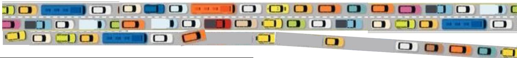
Auxiliary lanes, or “exit-only lanes” begin at one freeway entrance and end at the next exit. Auxiliary lanes are often used for safer merging when the distance between highway exits is short, e.g. between 41st Ave and Bay Ave. The longer auxiliary lanes proposed for Hwy 1 (1 mile and 1.5 miles) will encourage some drivers to switch into those lanes during periods of congestion. When the lane ends, drivers merge back into the through-lane, causing delays that exacerbate traffic congestion.
